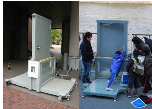
Evacuation Experiment by Use of Door Model (from Prof. Ishigaki's keynote lecture)
