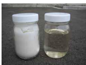
Fig.15 Produced Heavy Oil (Left) and Light Oil (Right) by Yufutsu GTL Plant
