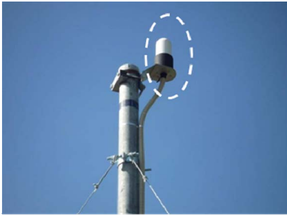
Fig.12 Doppler radar type rainfall gauge
