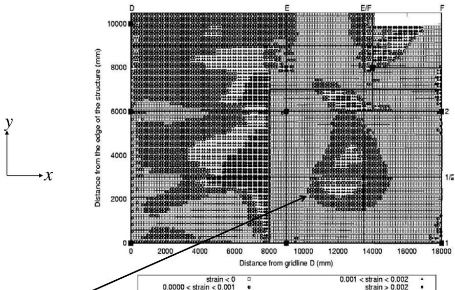
Compatibility enforced tensile strains in the y direction
