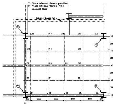
Test 3 - Transducer Positions for Measuring Vertical Deflections
