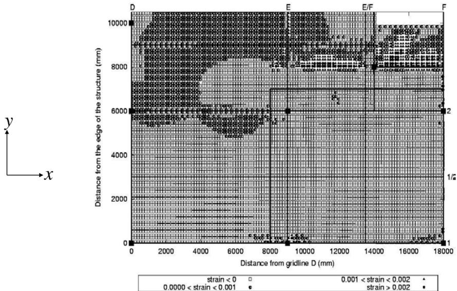
All of the slab in the fire compartment is under compression
